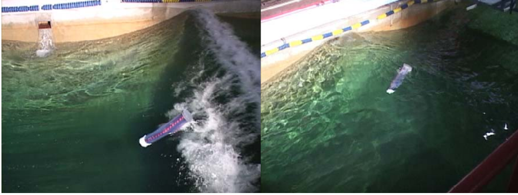
Figure 3.15: Two frames for Trial T, testing the large instrumented cylinder in the large wave tank.
