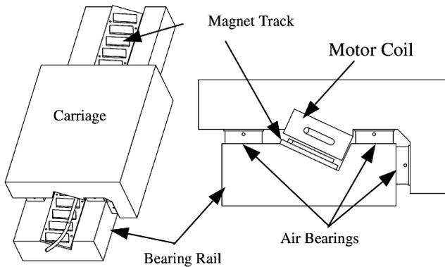
Fig. 1. Motor-preloaded-bearing concept where an iron-core open-face linear electric motor's permanent magnets are used to preload aerostatic bearings.
