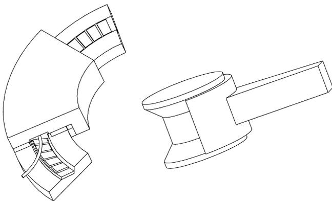
Fig. 2. Motor-preloaded-bearing angular motion design concepts where fundamentally the rotor is an arc segment. Left view shows an iron-core open-face rotary electric motor's permanent magnets are located on a conical surface and used to preload aerostatic bearings. Right view shows conical bearings with magnets that would be on a cylindrical surface.
