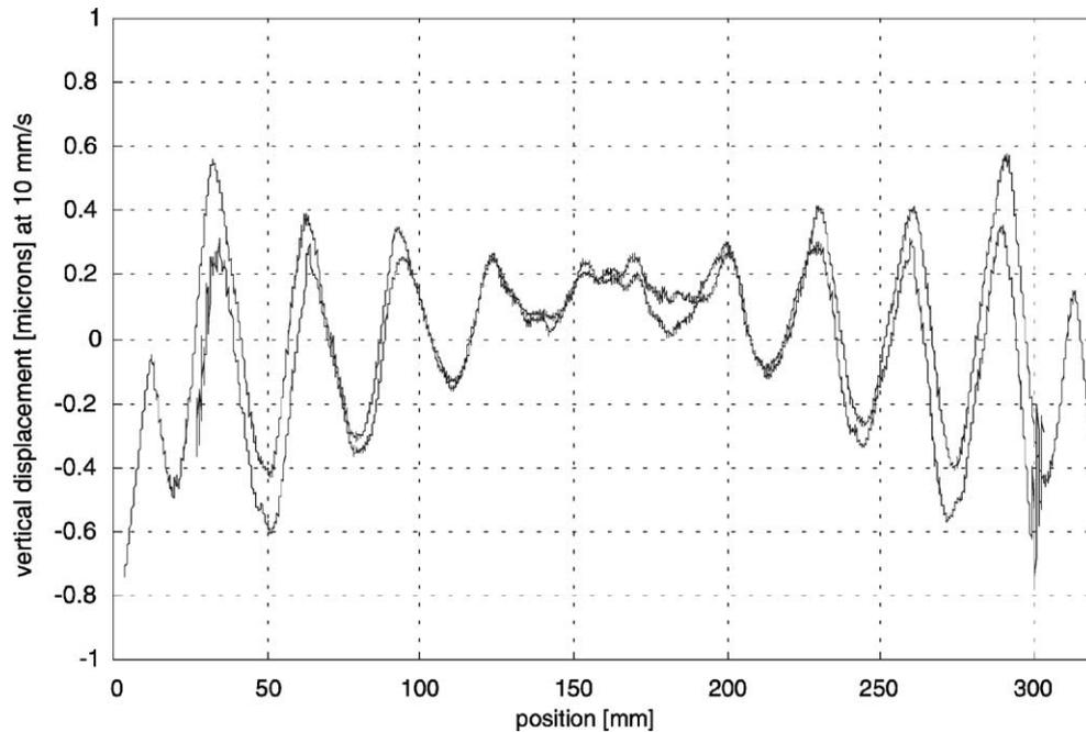
Fig. 16. Straightness measurements taken with a moving straightedge as shown in Fig. 10; hence, straightness includes product of pitch error and axial distance from center of carriage.
