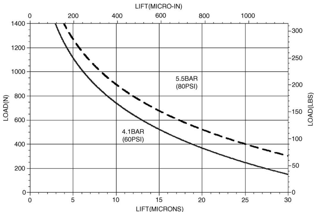
Fig. 3. Load vs. gap height and pressure for 50 mm  $\times$  100 mm commercially available porous graphite air bearing pad ([www.newwaybearings.com](http://www.newwaybearings.com)).
