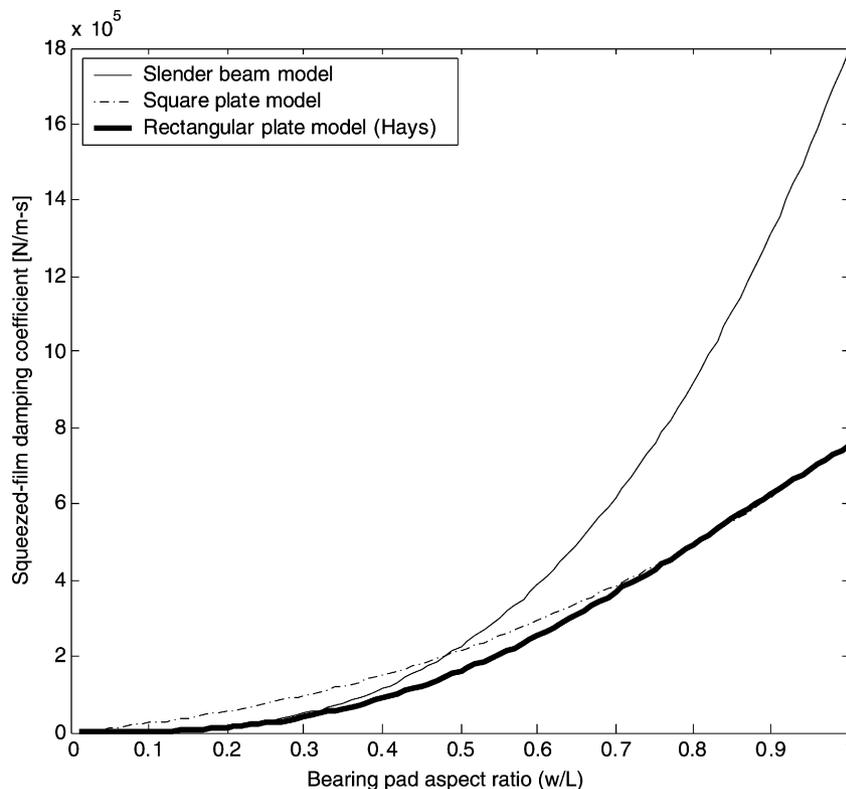
Fig. 4. Squeezed-film damping coefficients predicted by slender plate, square plate, and rectangular plate models.
