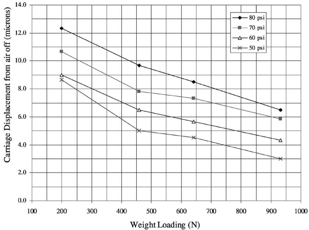
Fig. 11. Average displacement of the carriage when the air is turned on.
