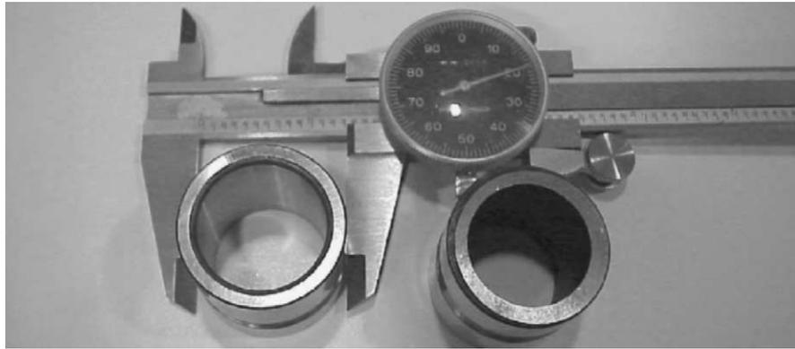
Fig. 18. Test parts ground on the bench level prototype system. Part: roller bearing inner ring; material: AISI 52100; hardness: 57–62 Rc; maximum stock removal: 0.300 mm on diameter. Required process: grind the bore diameter and maintain 0.4 Ra or better surface finish and 0.005 mm or less taper and straightness. Incoming part condition: back face (locating surface) and OD were ground.
