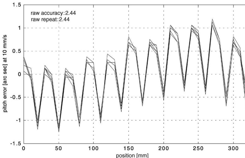
Fig. 15. Pitch motion of the carriage; the period is equal to the magnet pitch.
