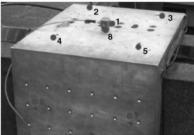
Fig. 12. The carriage and the 8 points used for modal analysis. Point 1 is the impact point, and Points 2–7 are the measurement points.
