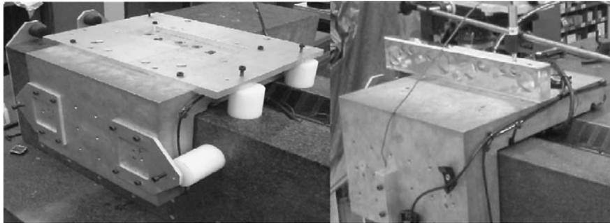
Fig. 10. Bench level prototype system with bearings being replicated in-place, and during metrology tests.
