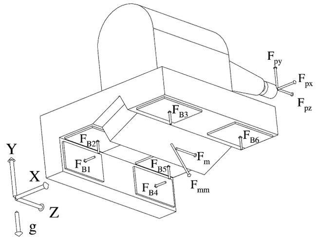
Fig. 5. Generalized forces on the carriage; note that the mass of the carriage and its location ( $m_c, x_c, y_c, z_c$ ) and the spindle ( $m_s, x_s, y_s, z_s$ ) are not shown.
