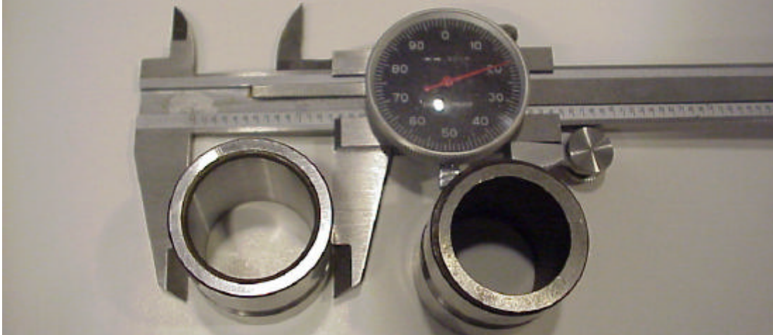
Fig. 15 Test parts ground on the bench level prototype system. Part: roller bearing inner ring. Material: AISI 52100. Hardness: 57-62 Rc. Maximum stock removal : 0.300 mm on diameter. Required process: Grind the bore diameter and maintain 0.4 Ra or better surface finish and 0.005 mm or less taper and straightness. Incoming part condition: Back face (locating surface) and OD were ground.
