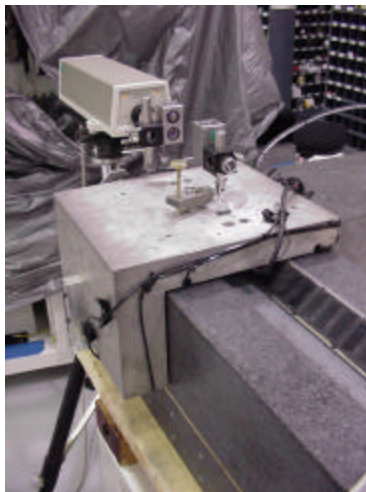
The basic setup for the pitch, yaw, and accuracy measurements. A laser and a variety of optics was used to make each measurement.
