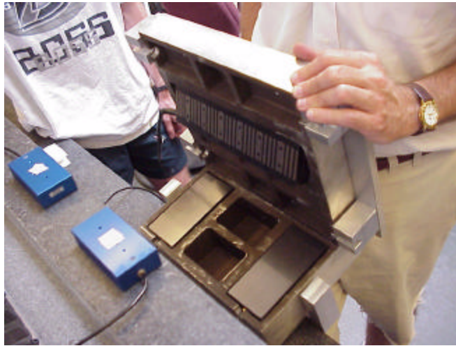
Figure A.6 The side bearings placed in their pockets before the carriage is put on the way.
