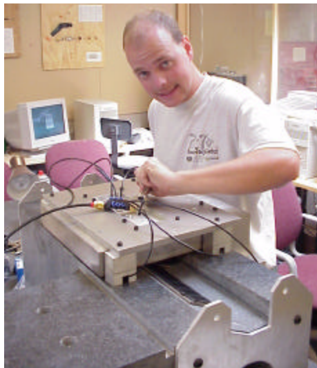
Figure A.7 Roger lowering the motor down onto the shim stock.
