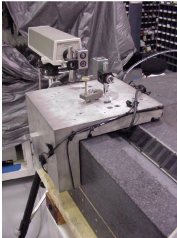
Figure A.10 The pitch measurement setup.
