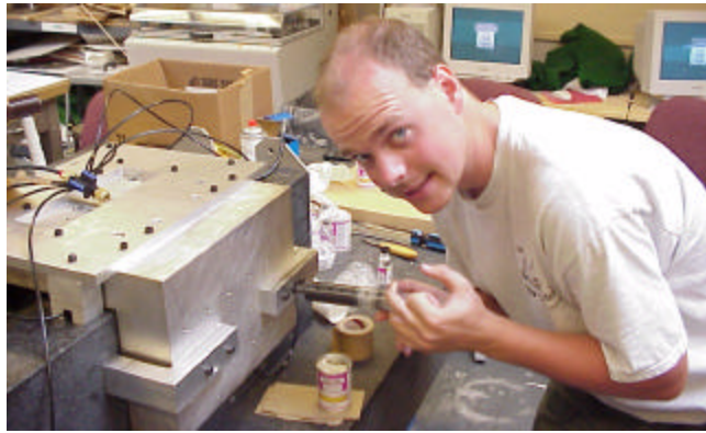
Figure A.9 Roger injecting epoxy into one of the side pockets.
