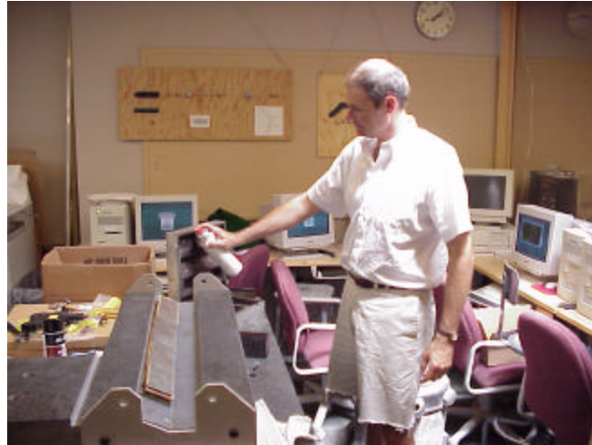
Figure A.3 Drew Devitt (Newway Bearings) degreasing the way.
