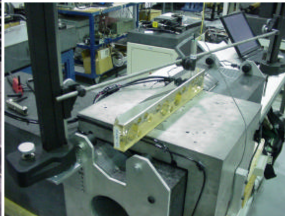
The basic setup for the vertical straightness measurement. The probe is suspended above the straight edge on the carriage.
