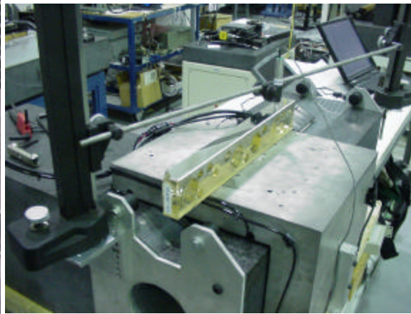
The basic setup for the vertical straightness measurement. The probe is suspended above the straight edge on the carriage.
